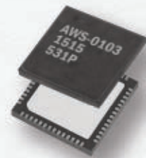
Surface mount 7x7 mm QFN
