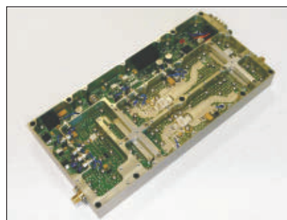
▲ Fig. 10 50 W, 0.5 to 2.5 GHz power amplifier.
